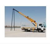
Submersible Pump - Pipe Dismantling Lifting Crane
